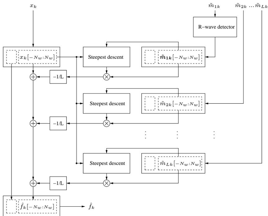
Figure 1: Diagram of the multichannel adaptive filter.
